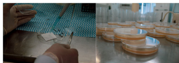
Figure 3 - Samples of bioactive packaging being prepared for the characterization of antimicrobial activity, being: (a) Addition of the microorganism in the packaging; (b) Culture medium
