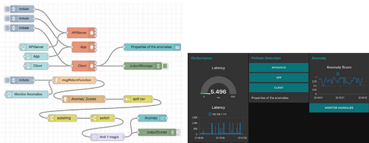
Figure 9 - Breakdown of node flows in the drag-and-drop implementation of Node-Red in the implementation and the dashboards produced to the user
