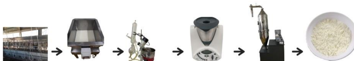
Figure 1 – Process for obtaining sheep's milk powder
