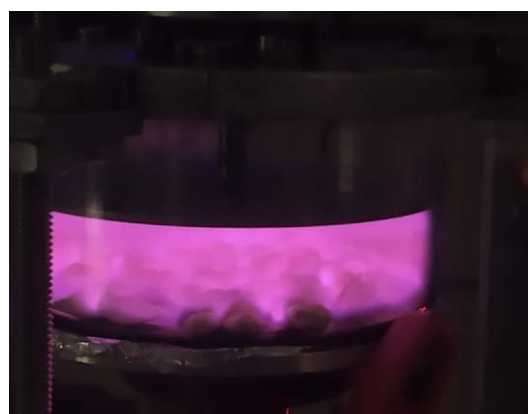
Figure 1 - (A) Schematic of the experimental setup used to treat 'Carrizo' citrange seeds with nitrogen plasma; (B) Photograph of the reactor under operating conditions
