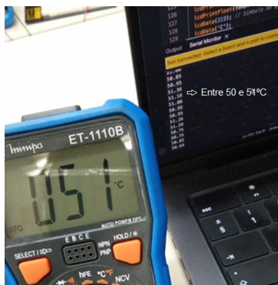
Figure 11 – Comparison of the measurement by Arduino and the “Reference System”
