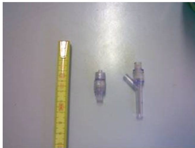
Figure 1: Heparin check valves compared with a tape meter (first on the left).
